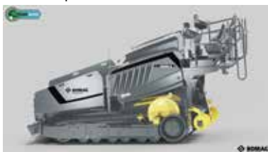
CR paver with the frame raised
