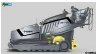
CR paver with the frame lowered
